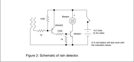
A narrow zig-zag gap is cut in the foil to electrically separate the two lead wires. The rain drops bridge the gap causing conduction which is sensed by the circuit shown in fig. 2.
